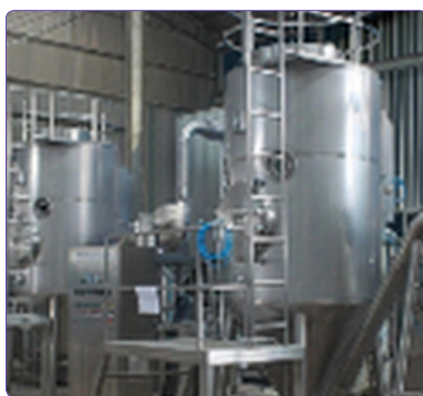
Hyundai Elevator Evaporative condensation treatment (100m 3 /day)
